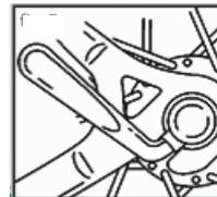
**(4)** Then, insert the wheel into the frame dropouts and pull it all the way in to the dropouts.
